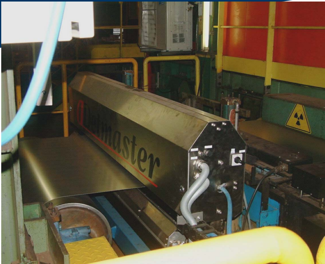
Picture 1 Detmaster 1300 MPH system installed on a Tin Plating Line No. 3
