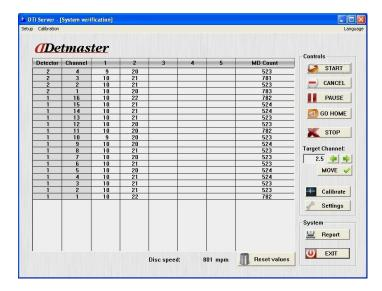
An advanced user interface with one-touch operation. Complete system check is carried out within 10 minutes. Real-time statistical window shows the detection rate and measured pinhole and hole size performance in micrometers.
