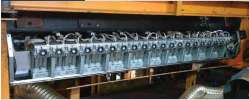
Detector beam with an array of array of 20 detector units. Beam is in off-line (roll-out) position with covers open.
